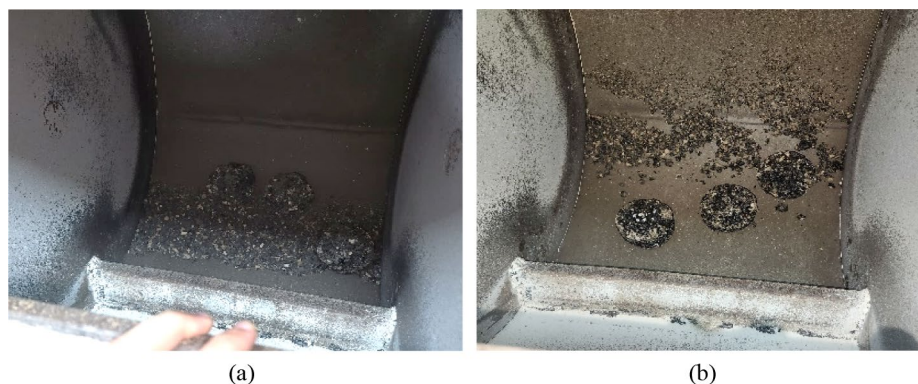
Figure 11. Porous asphalt mixtures after 300 revolutions into Los Angeles machine (a) control mixtures, (b) modified mixtures.
